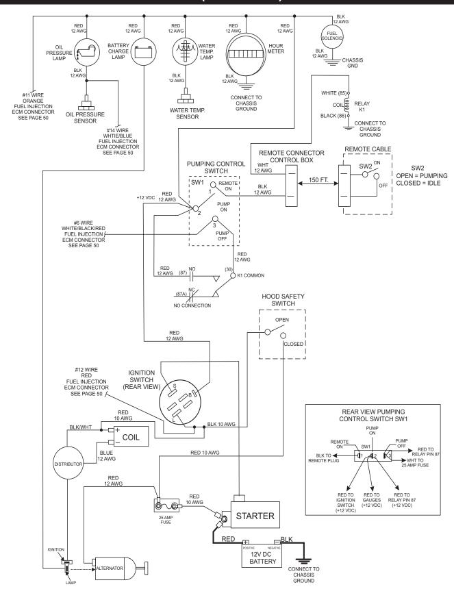
Figure 33. Wiring Diagram
